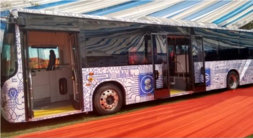
Electric buses with super capacitors that get charged at bus-stops through contactless technology could be seen at Indian roads, if the Purta concept sees commercial production.
